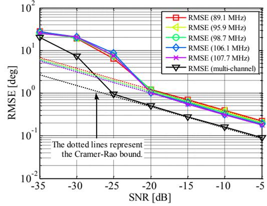
**Figure 2.** The RMSE of the single-channel and the multi-channel based PBR according to the SNR of target echo signal.
