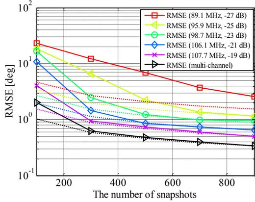
**Figure 3.** The RMSE of the single-channel and the multi-channel based PBR according to the number of snapshots.
