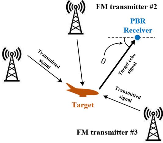
**Figure 1. The multi-static geometry of the PBR system.**
